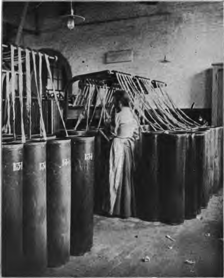
RECEIVING THE "SLIVER" AT THE BACK OF THE DRAWING FRAME.
